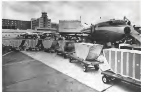
CARGO CAPSULES , built by Lockheed Aircraft, are loaded by Pan American World Airways Boeing 707-120 jet transport at Miami in preparation for its cargo service to San Juan, Puerto Rico. Aerial view. The system can load and off-load cargo in 20 min.
